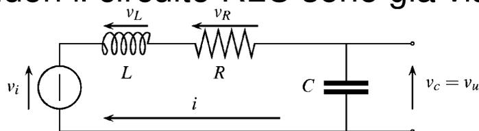
$$\text{con } i(0^+) = i_0, \quad v_u(0^+) = e_0, \quad v_i(t) = \begin{cases} 0 & \text{se } t < 0 \\ v_0 & \text{se } t \geq 0 \end{cases}$$
