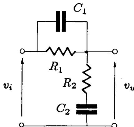
$$\Rightarrow G(s) = \frac{V_u(s)}{V_i(s)} = \frac{\frac{1}{sC_2} + R_2}{\frac{1}{sC_1 + (1/R_1)} + \frac{1}{sC_2} + R_2}$$
