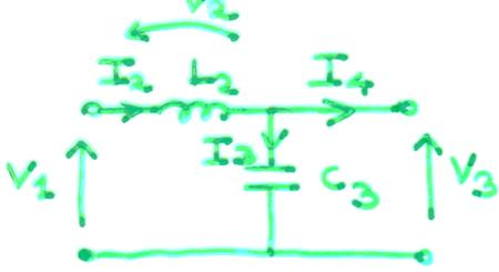
$$I_2 = \frac{V_2}{sL_2} = \frac{V_1 - V_3}{sL_2}$$
