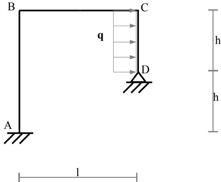
$$l = 2 \text{ m}, h = 1 \text{ m}, q = 20 \text{ kN/m},$$
