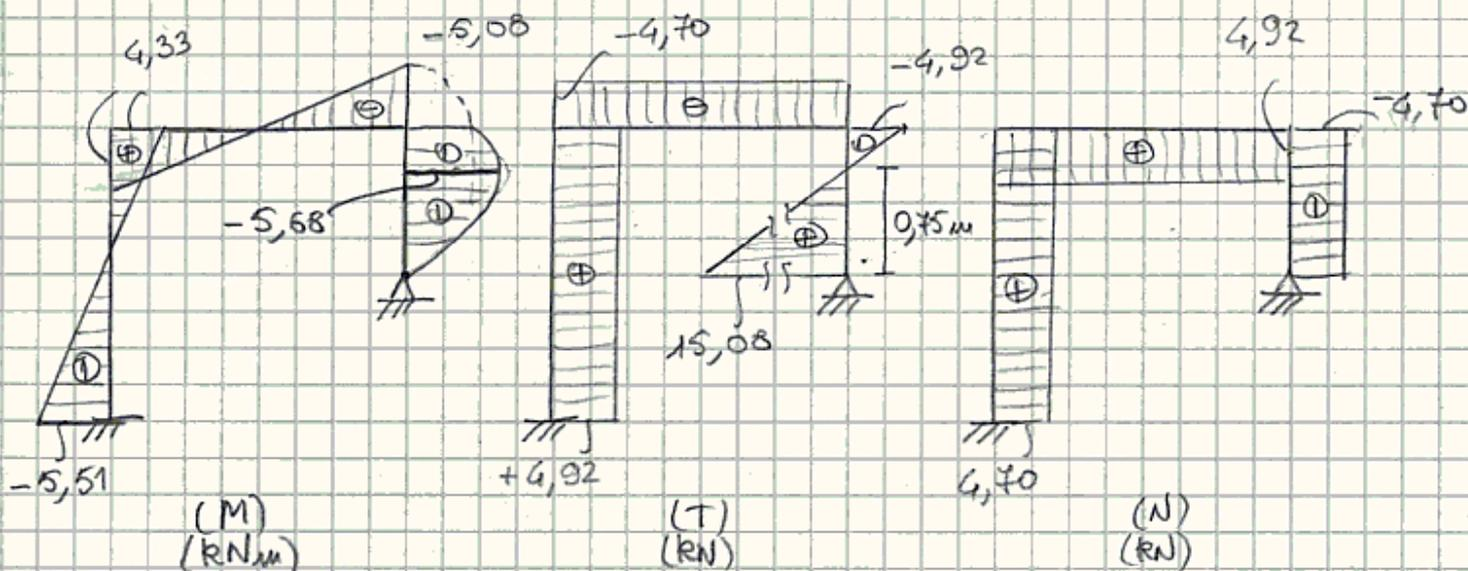
2) Progetto:  $W_{I, \geq} \frac{M_{max}}{\sigma_{amm}} = \frac{5,68 \cdot 10^3}{240 \cdot 10^6} \cdot 10^8 \text{ cm}^3 = 23,66 \text{ cm}^3$
