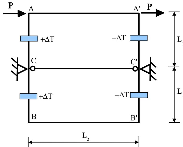
$$L_1 = 2 \text{ m}, L_2 = 4 \text{ m}, P = 50 \text{ kN}$$
