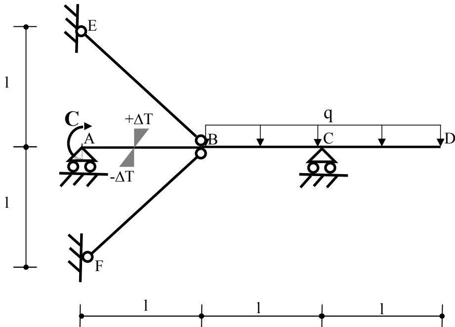
$$l = 1 \text{ m}, q = 2 \text{ t/m}, C = 4 \text{ tm}, \\ E = 2.1 \cdot 10^6 \text{ kg/cm}^2, \alpha = 10^{-5} \text{ }^{\circ}\text{C}^{-1}, \Delta T = 20 \text{ }^{\circ}\text{C}$$
