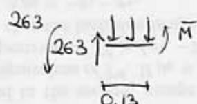
$$\begin{aligned} M &= -263 + 263 \cdot 0.13 - 2000 \cdot 0.13^2 \\ &= -246 \text{ kg m} \end{aligned}$$
