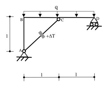
$$\begin{split} 1 &= 2 \text{ m, } q = 2 \text{ t/m,} \\ \sigma_{AMM} &= 2400 \text{ kg/cm}^2 \text{ , E} = 2.1 \text{ } 10^6 \text{ kg/cm}^2 \\ \Delta T &= 20 ^{\circ}\text{C, } \alpha = 10^{-5} \text{ } ^{\circ}\text{C}^{-1} \end{split}$$
