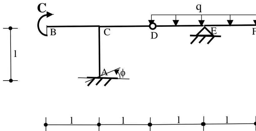
$$l = 1 \text{ m}, q = 1 \text{ t/m}, C = 2ql^2, \sigma_{AMM} = 2400 \text{ kg/cm}^2 \\ E = 2.1 \cdot 10^6 \text{ kg/cm}^2, \phi = 0.2^\circ$$
